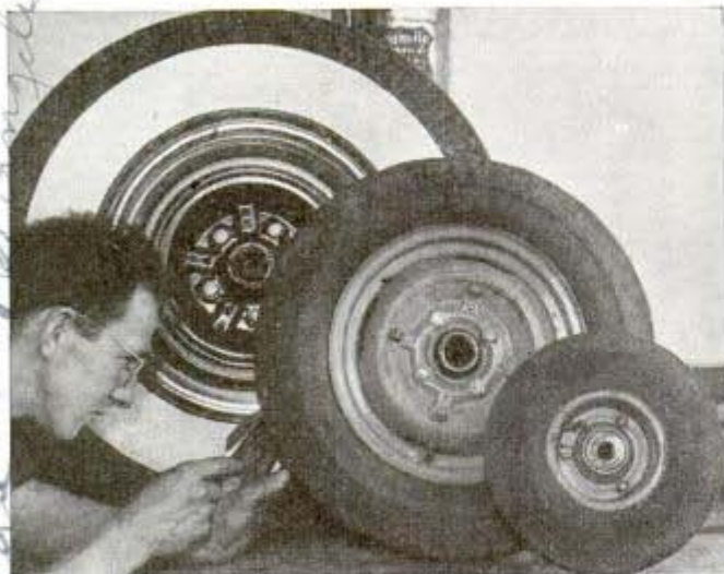
Examine tires for nails in the treads. They may not cause an immediate puncture, but will result in damage unless pulled out
